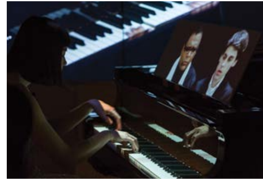
XIAO XIAO'S MirrorFugue is a technologically enhanced player piano that captures the facial expressions, body movements and hand positions of the musician in a projected reflection.
